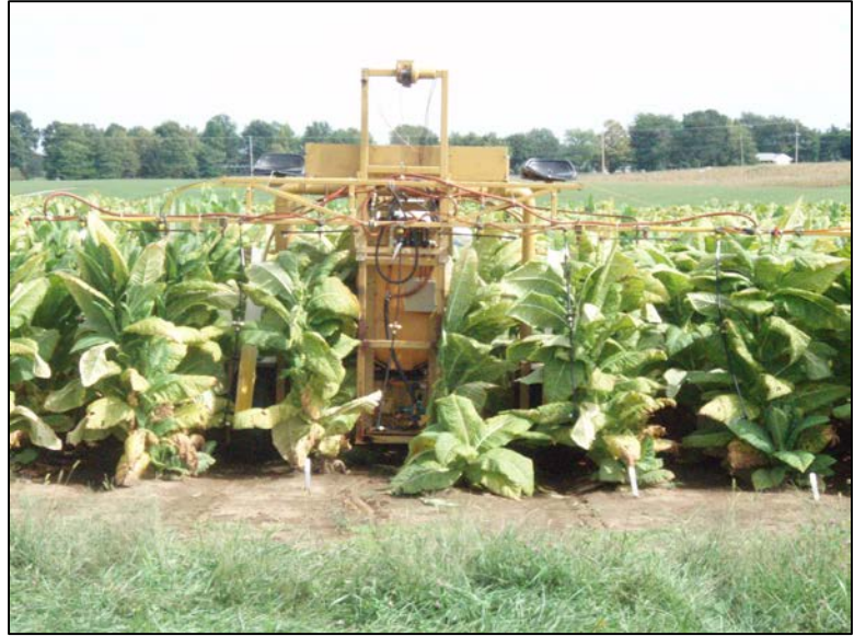
Figure 5: Spray application with a high clearance tractor
